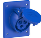
*CEE-flanged socket sloping (80x97mm) 16A 3p 6h IP44/IP54 (413-6f8)
